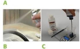
A. To grant adhesion, you may use the water-based Adhesion Promoter, mixed with 7-8% Eco-Crosslinker or 1-3% of Crosslinker AZ5. The more powerful, solvent based Extra Adhesion may also be used but it is less environmentally friendly than the waterbased. Use masking tape to cover any part of the steering wheel not to be painted. Apply by spray to create a light coat. Dry with a hairdryer.
