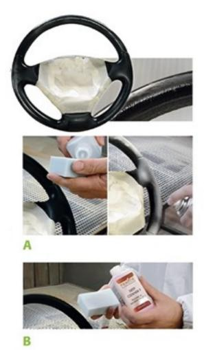
A. Remove surface dirt by cleaning the steering wheel with a **Stain Eraser Sponge** soaked in **Power Cleaner**diluted with water, rubbing with circular movements. Remove any excess product with absorbent paper or clean, dry cloth and leave to dry.
