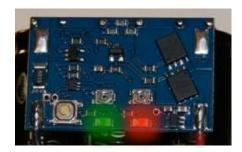
You are now ready to fly. Bare in mind that the high capacity capacitors charge logarithmically and it may take up an additional minute before the capacitors reach maximum charge.
