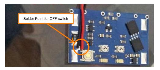
2. The external "ON" switch is installed between the positive (+) LiPo and positive (+) output solder points as depicted below:
