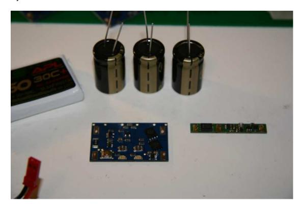
The assembly instructions are separated into specific sets for NC (Capacitor) and NL (LiPo) configurations. It is possible to assemble the unit for NC and then later switch to NL. Switching from NL to NC is not recommended due to the required removal of the balancing (See the *NL* (*LiPo*) assembly instructions section for more details).
