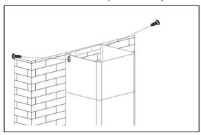
Remove all blue protective film on chimney and cooker hood, the installation is now finished.
