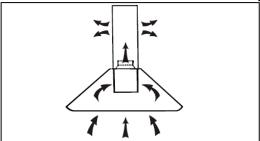
Activated carbon filter can be used to trap odours.
