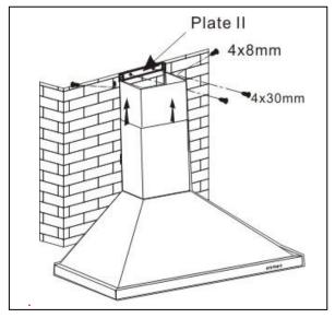
Use 2pcs ST4x8mm screws to attach lower and upper chimney together, do not fasten screws too much, make sure *upper decorative chimney* can be telescopically adjusted after assembled.
