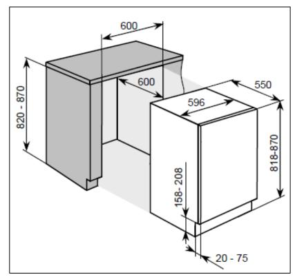
• The appliance must be stood on a level floor. You can use the levelling feet to take into account any minor unevenness in the floor.
