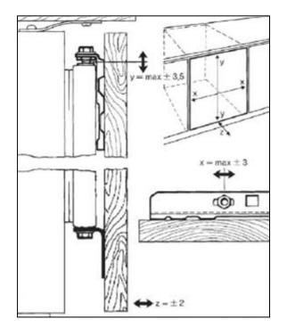
c) Use a screwdriver to adjust the gap on the lower section of the adjusting bolts. The gap should be set to approximately 9 mm (as shown in the above drawing).
