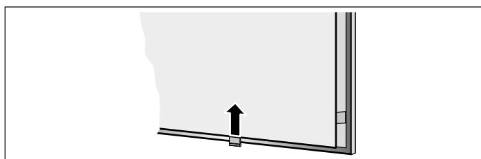
4. Take the metal grease filter out of the holder.
