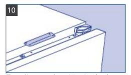
The appliance must be positioned so that the top bracket is flush with the underside of the work surface and flush with the her units. See 'Adjusting the height and level of the appliance' on page 3.
