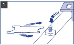
Remove the two plastic plugs on the top of the door and insert the double-ended bolts.
