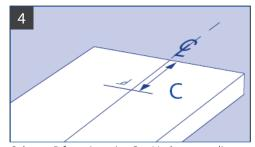
Subtract B from A to give C=. Mark a centre line down the length of the rear of the Cabinet Door. Measure the disatnce C from the top of the door and mark a line 90° to the centre line.
