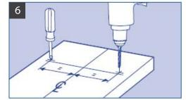
Mark the centre of the drill holes using a bradaw. I Remove the brackets. Using a 3mm drill bit, drill a hole to a depth of 5 - 8mm.
