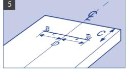
Drawer a line the length of D on the rear of the door. Ensure that it is centred over the centre line. Place two of the brackets so that the bottom of each bracket is in line with the horizontal mark.
