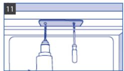
Open the appliance door. Use two screws and a drill bit that are appropriate to your work suface, mark and drill through the bracket into the underside of the work surface. Screw the brackets to the work suface.
