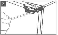
With the door closed remove the screws on the outside of the hinges. Start with the top hinge.
