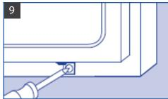
Fit the two remaining right-angled brackets to the bottom of the appliance door using the two bolts provided. Mark the hole centres on the outer cabinet door and remove it. Using a 3mm drill bit, drill a hole to a depth of 5-8. Refit the outer cabinet door and screw the brackets in place.
