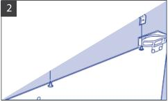
Place two of the right-angled brackets on the bolts and secure with the domed headed nuts. Measure the distance between the centres of the bolts. D=
