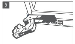
Repeat with the other hinge. Replace the cabinet blanking plates. Replace the door and re-attach the hinges.
