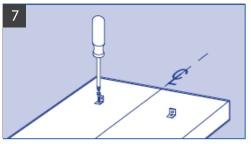
Using the screws provided, screw the brackets into place.
