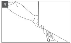
Supporting the bottom of the door as you do so. Be careful with the hinges. Remove the door.
