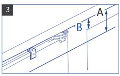
Measure from the underside of the work surface to the bottom of the right angled bracket. A= Next measure from the underside of the work surface to the top of the other unit doors. B=
