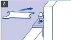
Fit the outer cabinet door onto the two bolts at the top of the appliance door and check that it is level with the other cabinet doors. Tighten the domed headed nuts to secure the backets.
