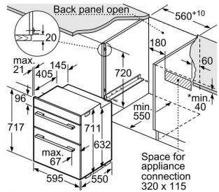
\* For installation under an induction hob, min. 50 measurements in mm
