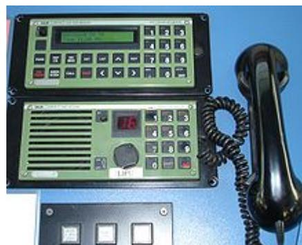
**Figure 1. A Ship's VHF Radio**
