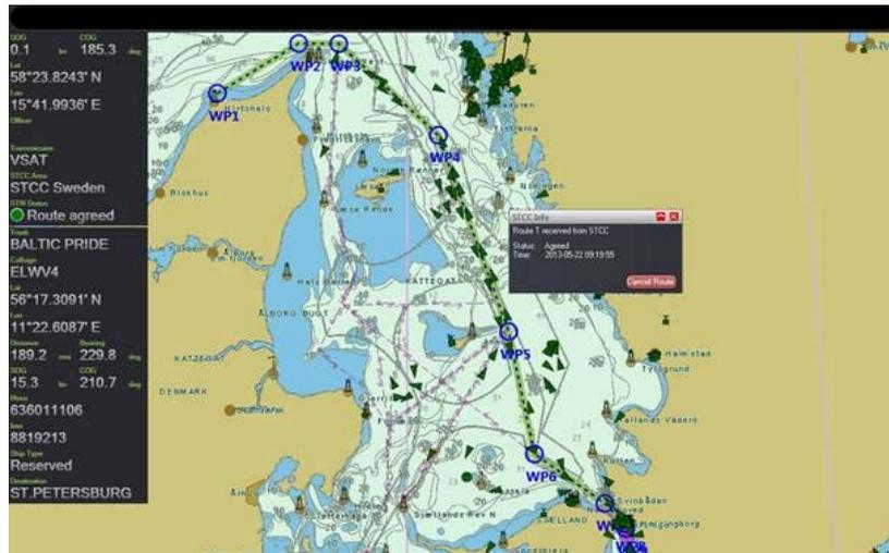
Figure 1. A "green" agreed route between the shore traffic control and the vessel in the MONALISA system, here in the SAAB prototype platform. Source: MONALISA Project Reports
