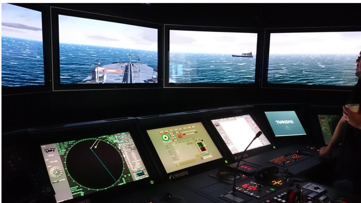
Gothenburg Transas bridge simulator looking at overtaking the vessel controlled in the Kongsberg bridge simulator in Gijon.
