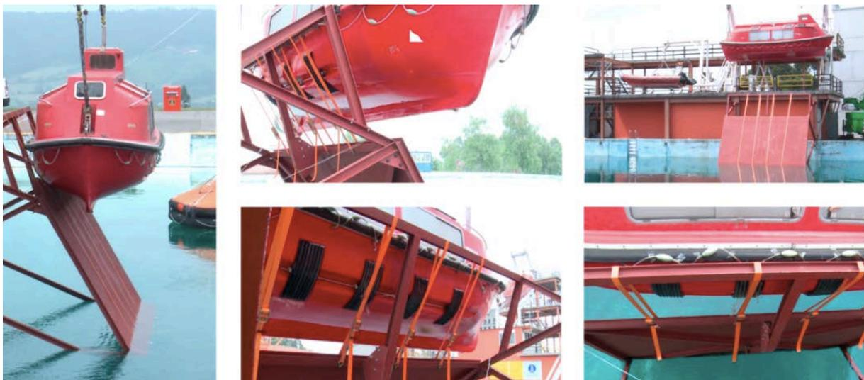
*Figure 5. Test with straps and sliding pads done during the MONALISA, SES project (SES, pilot application).
