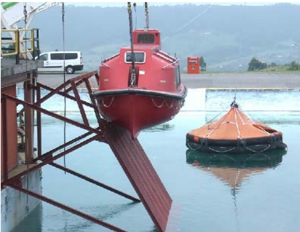
*Figure 4. Tests done in basin at Centro Jovellanos in Gijon (SES, launching and recovery system design). Reprinted with permission.*
