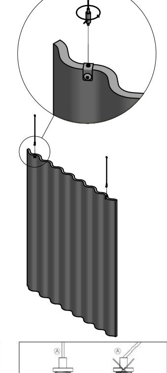
A. Direction of wire and gripper must be in a straight line
