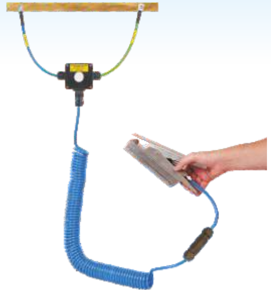
Bond-Rite CLAMP supplied with 2 conductor cable, junction box, clamp stowage pin and grounding leads. Circuit monitoring board and battery mounted inside clamp. Grounding bus-bar not supplied.
