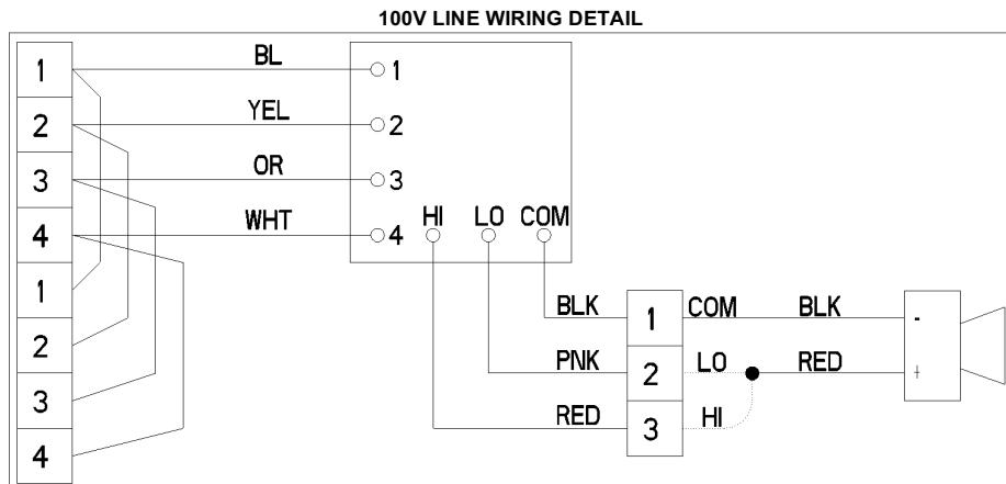
In the 100V line versions, the Exe chamber contains two 4-way terminal blocks (both numbered 1-4) for the 100V line connection and to allow a loop-in, loop-out facility. The chamber also contains a single 3-way terminal for selecting the 'hi' or 'lo' range of tappings. Connect the red +ve driver wire to the relevant terminal to select the required range. Do not power up the unit without the +ve driver wire connected to one of the available terminals. See table below for available tappings.
