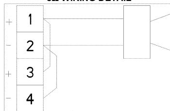
For the 8Ω versions, there is a single 4-way terminal block for direct connection to the driver wires as shown above.
