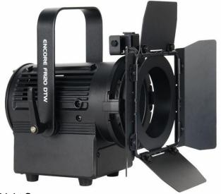
Part of the Encore stage lighting series, the Encore FR20 DTW lighting fixture is equipped with a 2-inch Fresnel lens and powered by a 17W warm white LED engine.
