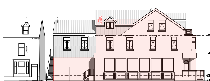
PROPOSED SIDE ELEVATION 1:100
