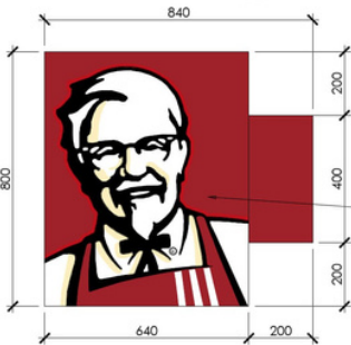
projecting sign detail scale - 1:10 @ A1 / 1:20 @ A3
