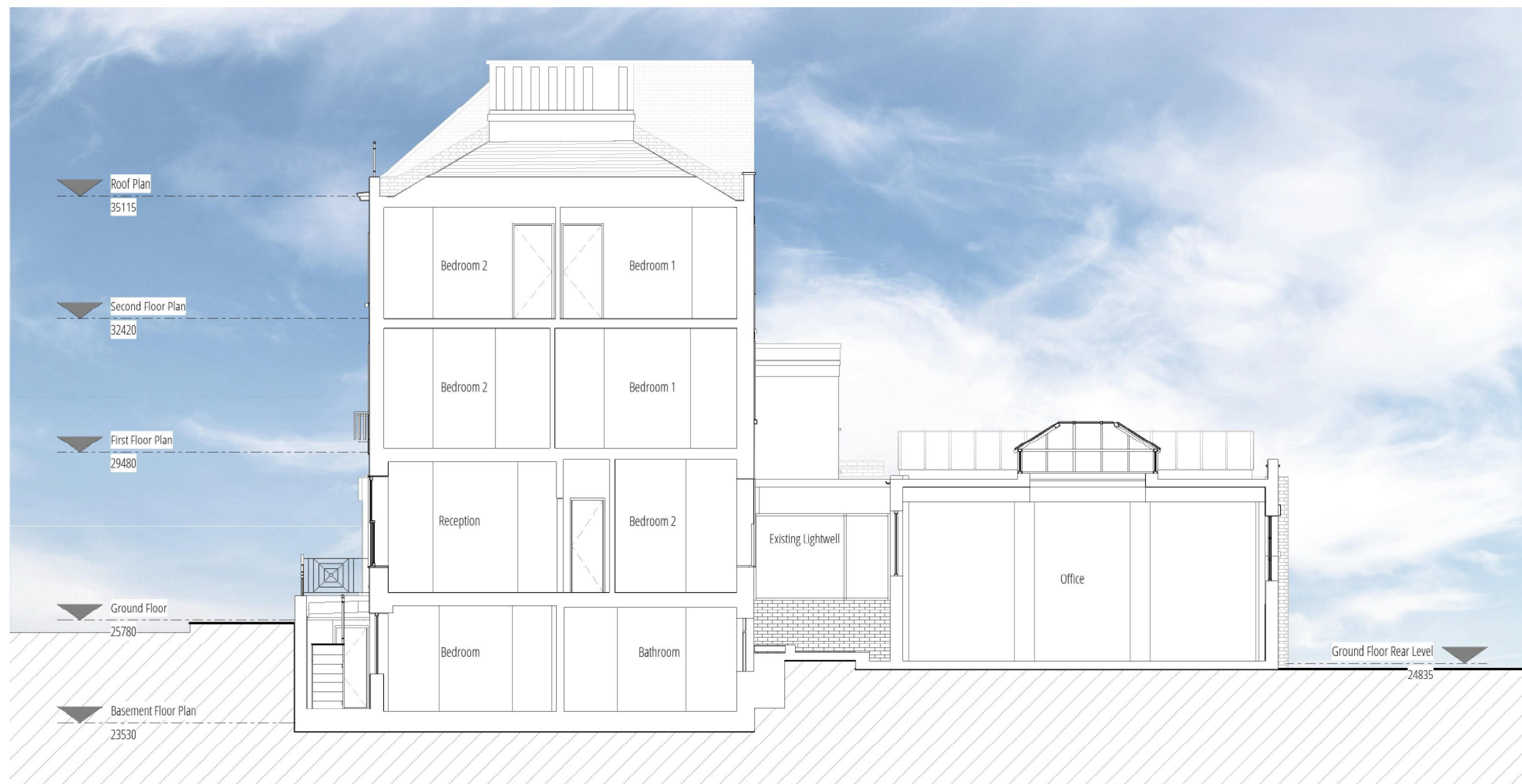
Fig 34 Existing Section DD' Scale 1:100 @A3
