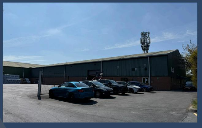
The subject property comprises a detached industrial/warehouse unit benefitting from a large tarmac yard area. The property comprises a steel portal framed construction with integral ground floor office accommodation. The unit is arranged across two connected bays in a L shaped configuration, surrounding a centra yard area. On the ground floor, there is a staff canteen and welfare area along with office space. There is first floor mezzanine storage in both bays.
