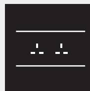
New perimeter trunking
