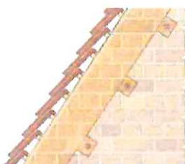
Restraining gable walls using mini retrofit purlins and BowTies
