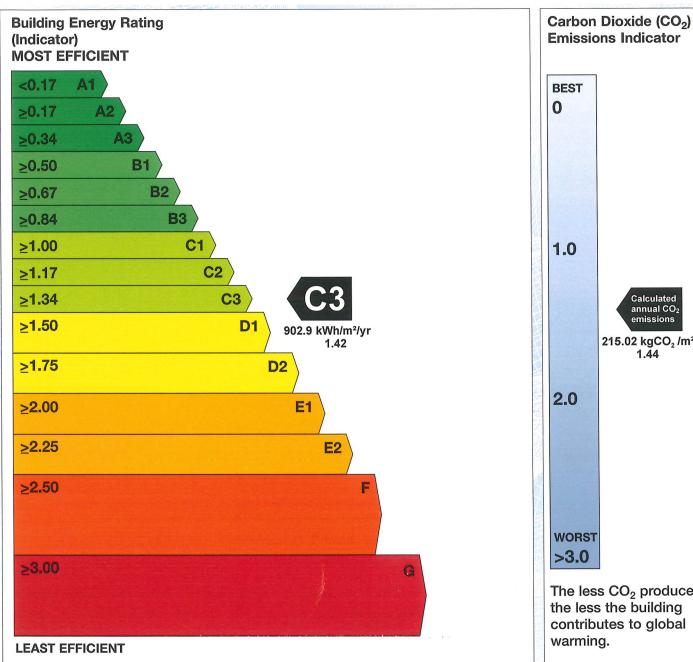
**Emissions Indicator** Calculated annual CO: emissions 215.02 kgCO<sub>2</sub> /m<sup>2</sup>/yr 1.44 The less CO<sub>2</sub> produced, the less the building contributes to global
