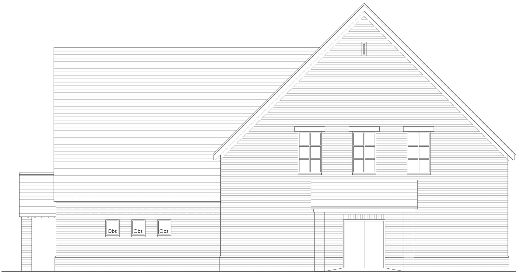
Side Elevation Obs = Obscure Glazing
