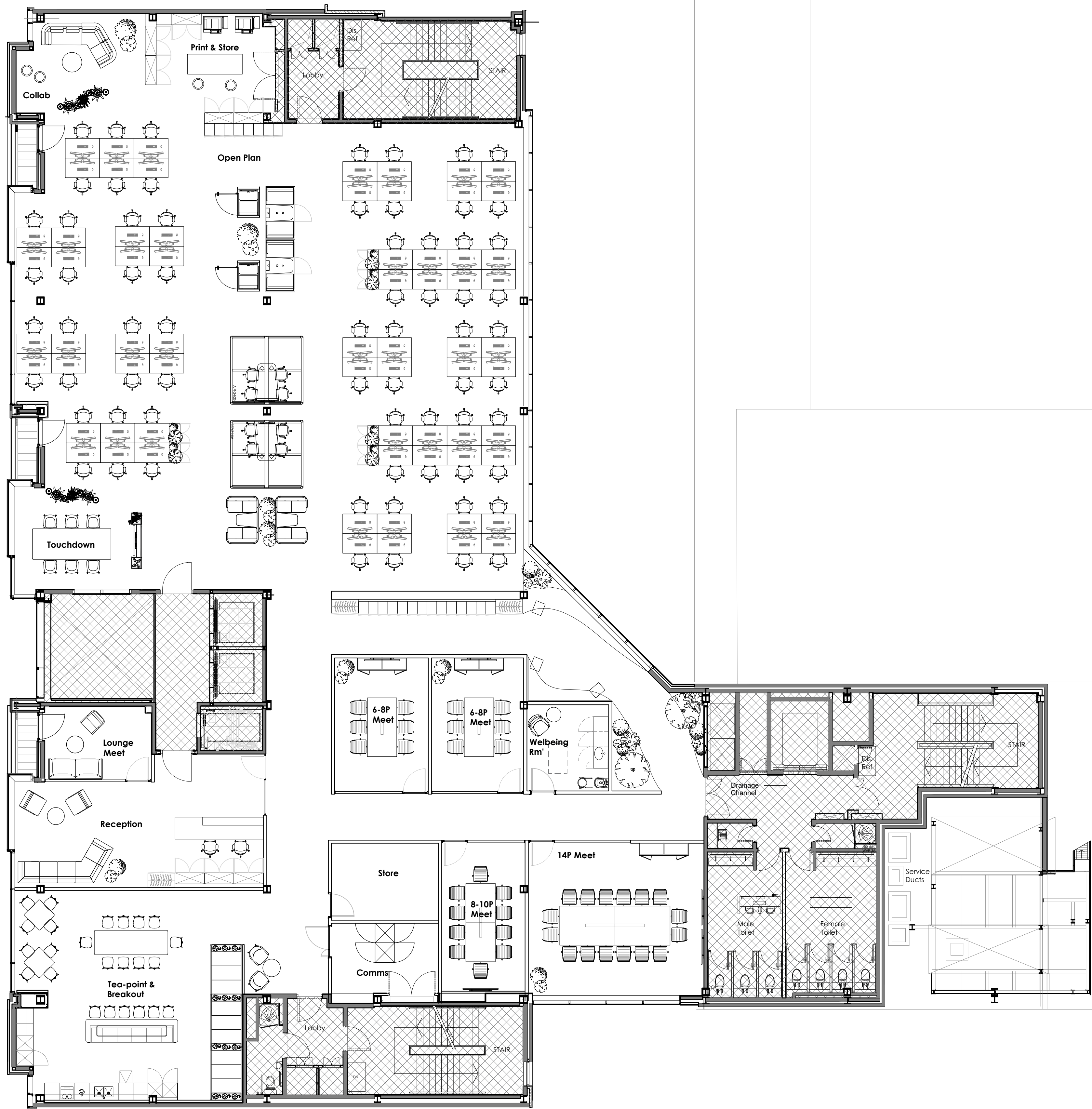
PROPOSED GENERAL ARRANGEMENT PLAN @ 1:100 Low-density 68no. workstations 0 1 2 3 4 5m Scale Bar @ 1:100
