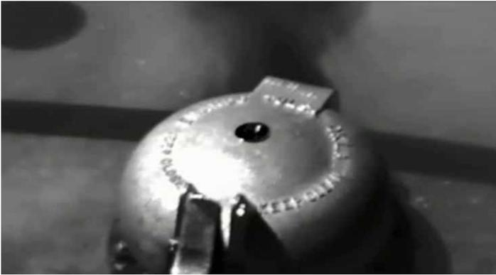
Optical gas camera shows methane leaking from thief hatch
