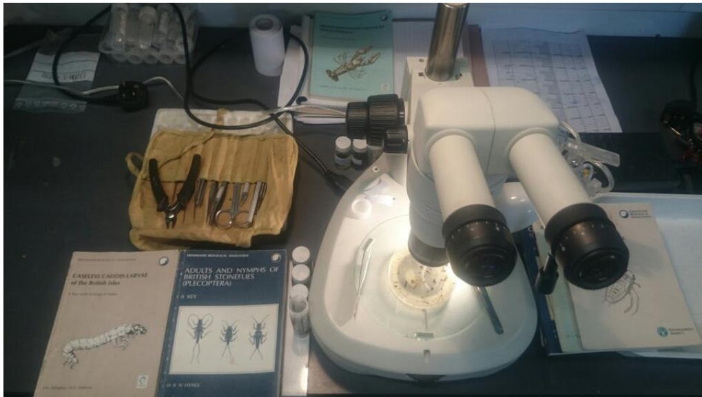
Plate 1 – Nikon SMZ1000 microscope with LED lighting used in the identification of samples
