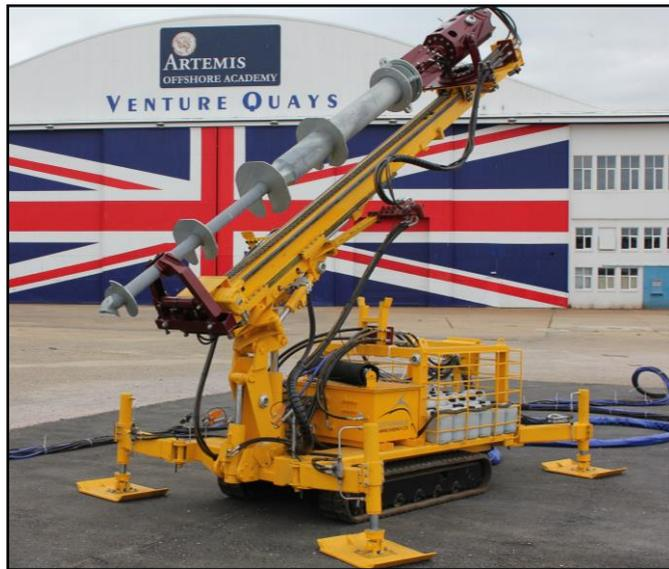
Fig 2: Loaded AROV in screw pile configuration prior to testing at Yarmouth
