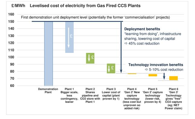
Levelised costs are in UK£ 2013, capital costs are +/- 40%( EPC \*1.4), discount rates are adjusted for risk (range 9-16%). Gas £24/ MWht and CO2 emission £31/te. All plants other than first demonstration plant are 860MW net output.
