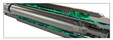
The final phase was to run the Oilenco wire roller brush to clear scale around the flow tube recess and brush the safety valve to remove any remaining debris. With all scale remedial work complete, final testing confirmed full reinstatement of the TRSSSV allowing operations to continue.
