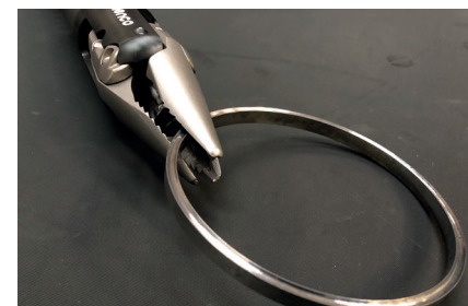
The Fishing Claw 'catching' an adaptor ring
