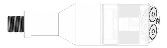
The Oilenco Eyeball Magnet is a dynamic fishing magnet, designed to allow full swivel and rotation of the magnet. This Ensures the magnetic face is free to swivel and locate loose objects within the well bore. The non-magnetic housing ensures maximum magnetic force is directed to the face.
