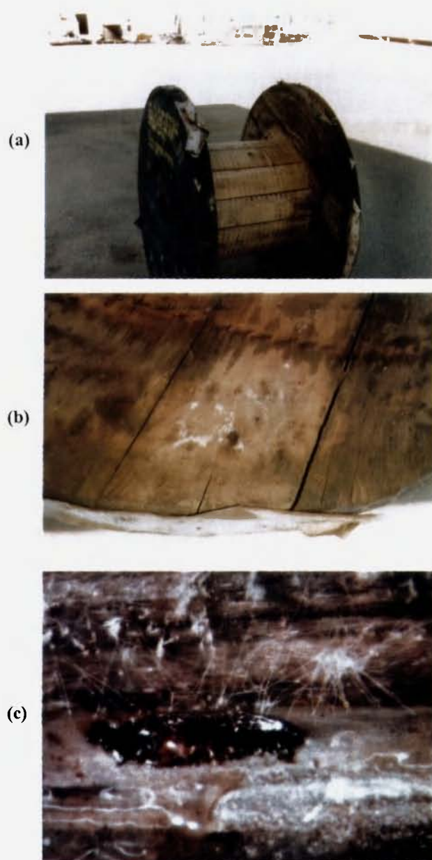
Fig. 4: (a) Wooden spool on which wire rope was stored. Pieces of paper are attached to rim edges. (b) Inside surface of wooden spool. White deposits are the result of fungal growth. (c) Light microscope photograph showing fungal mycelia attached directly to wire and associated with localized corrosion, 40X.
