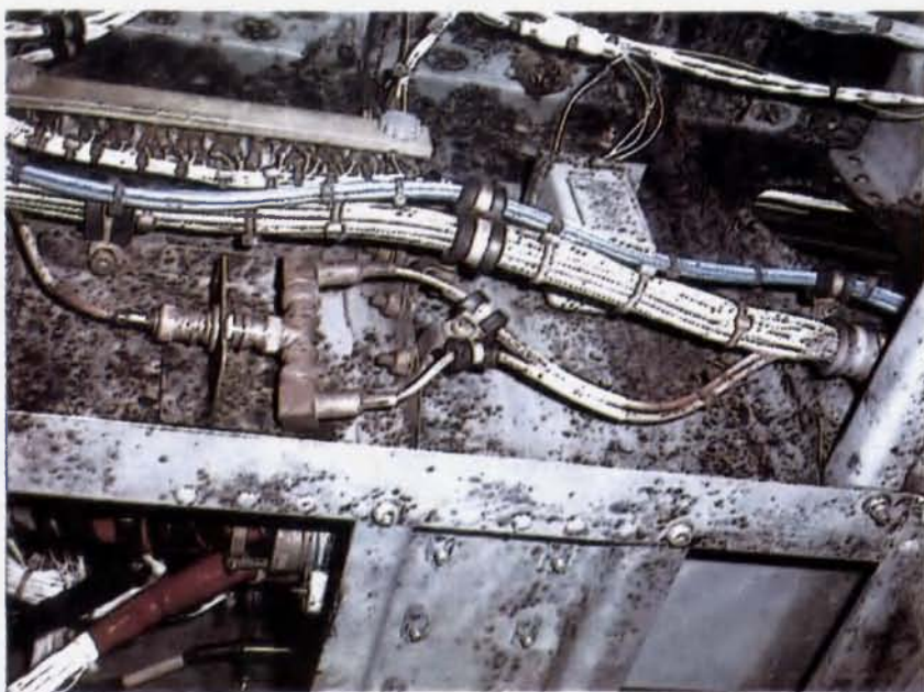
Fig. 2: Interior of helicopter with luxurious fungal growth on polyurethane paint.
