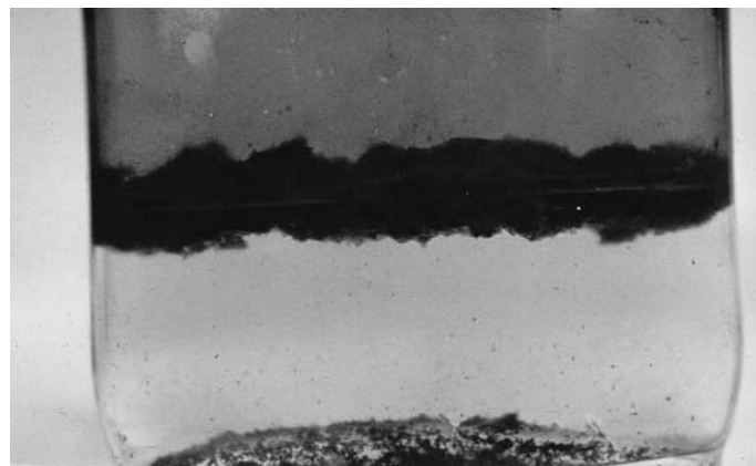
Figure 2 Invert emulsion layer forming in diesel fuel above biofilm which is growing at diesel:water interface.
