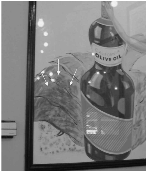
Fig. 1 Poster with mold colonization in lower left corner induced by cooling the glass below the dew point. Note the parabolic contour of the top edge (arrows) of the colonized area, corresponding to the conical discharge of cold air from an HVAC duct above the poster.
