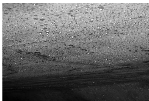
Figure 3 Snottites growth on the surface of a cement based lining material (Sample B)
