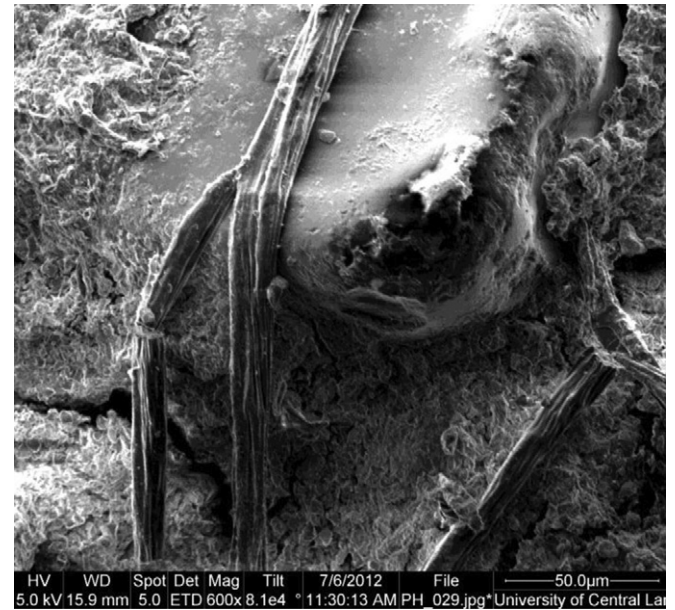
Fig. 6. SEM, secondary electron micrograph, surface view of revetment armour concrete surface, after 3 years exposure. This sample was not sputter coated, showing the filament in its natural condition. A branched mature filament can be seen growing over the exposed fine aggregate.
