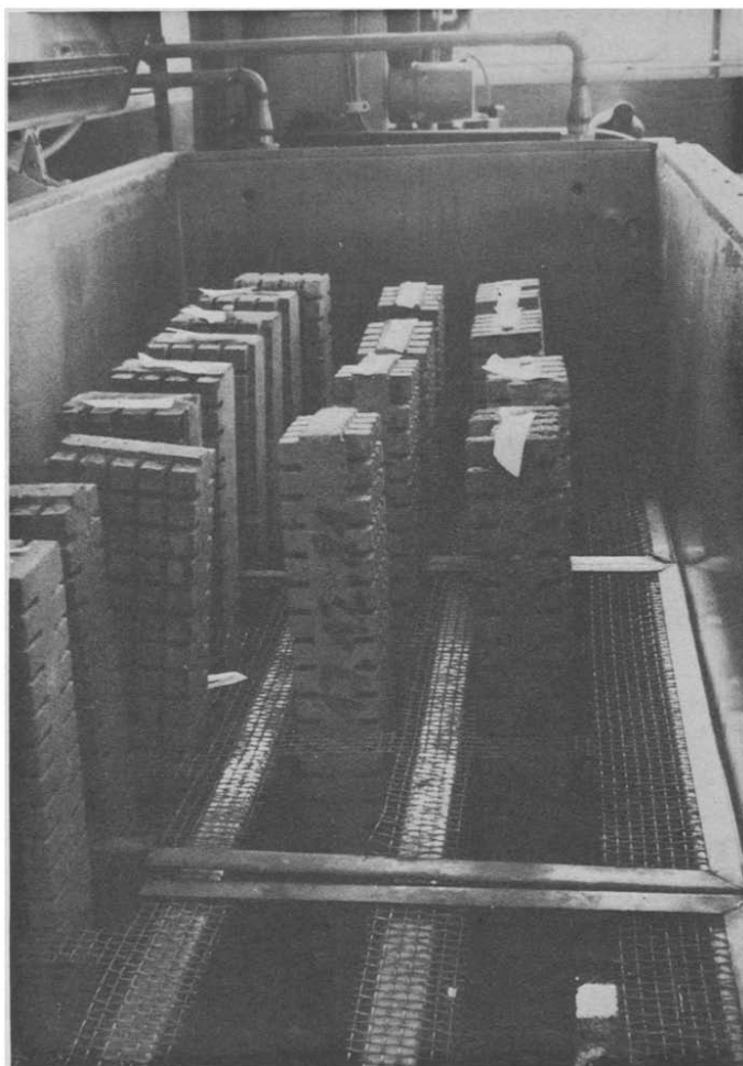
Fig. 2. Presawn concrete test blocks in the simulation chamber for biogenic sulphuric acid corrosion.
