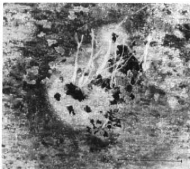
Fig. 5. Magnified part of corrosion site of an Al 7075 sample incubated at 30°C for 28 days in PYG-medium, inoculated with Penicillium sp. Bar: 1 mm
