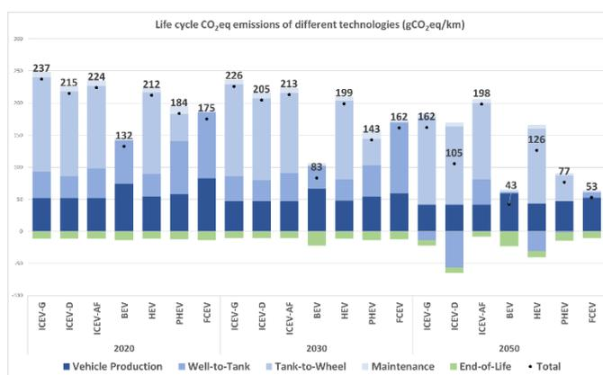
Figure 1: vehicle-specific LC CO<sub>2</sub>eq emissions for mid-size cars.
