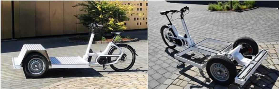
Figure 1: Commercial tricycle with checker plate on the left hand side and with a direct view onto the front end frame on the right hand side.
