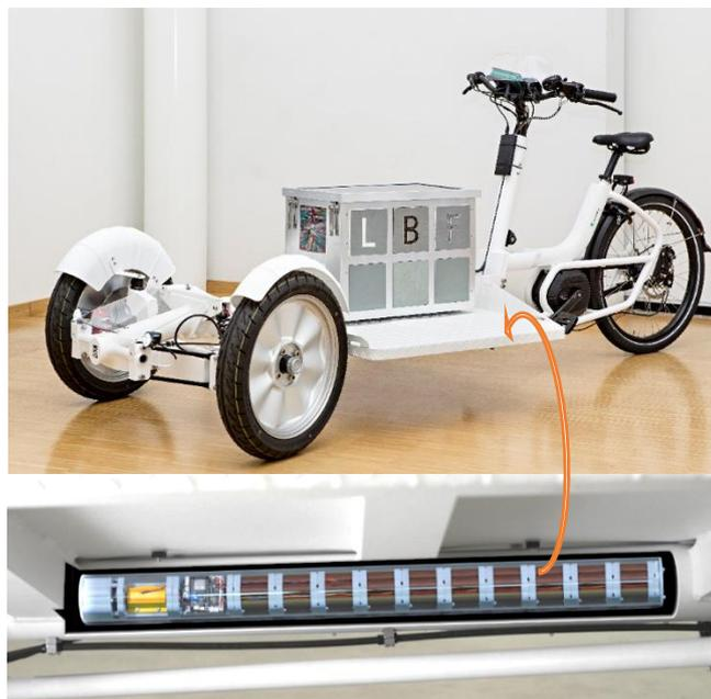
Figure 4: The modified cargo bike is shown on top and the TES, integrated in the frame tube under the checker plate, is arranged below.
