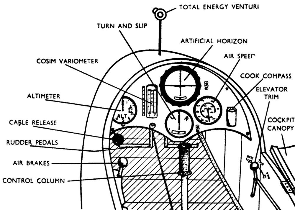
Fig. 3. The cockpit layout of a modern glider.
