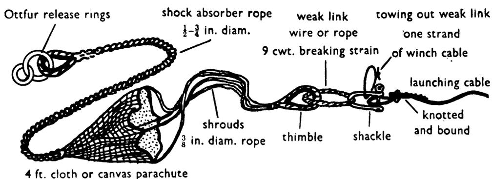
Fig. 4. The cable make-up.
