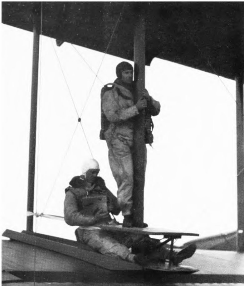
Parachute platform on wing of Vickers Virginia. (RAF Museum).
