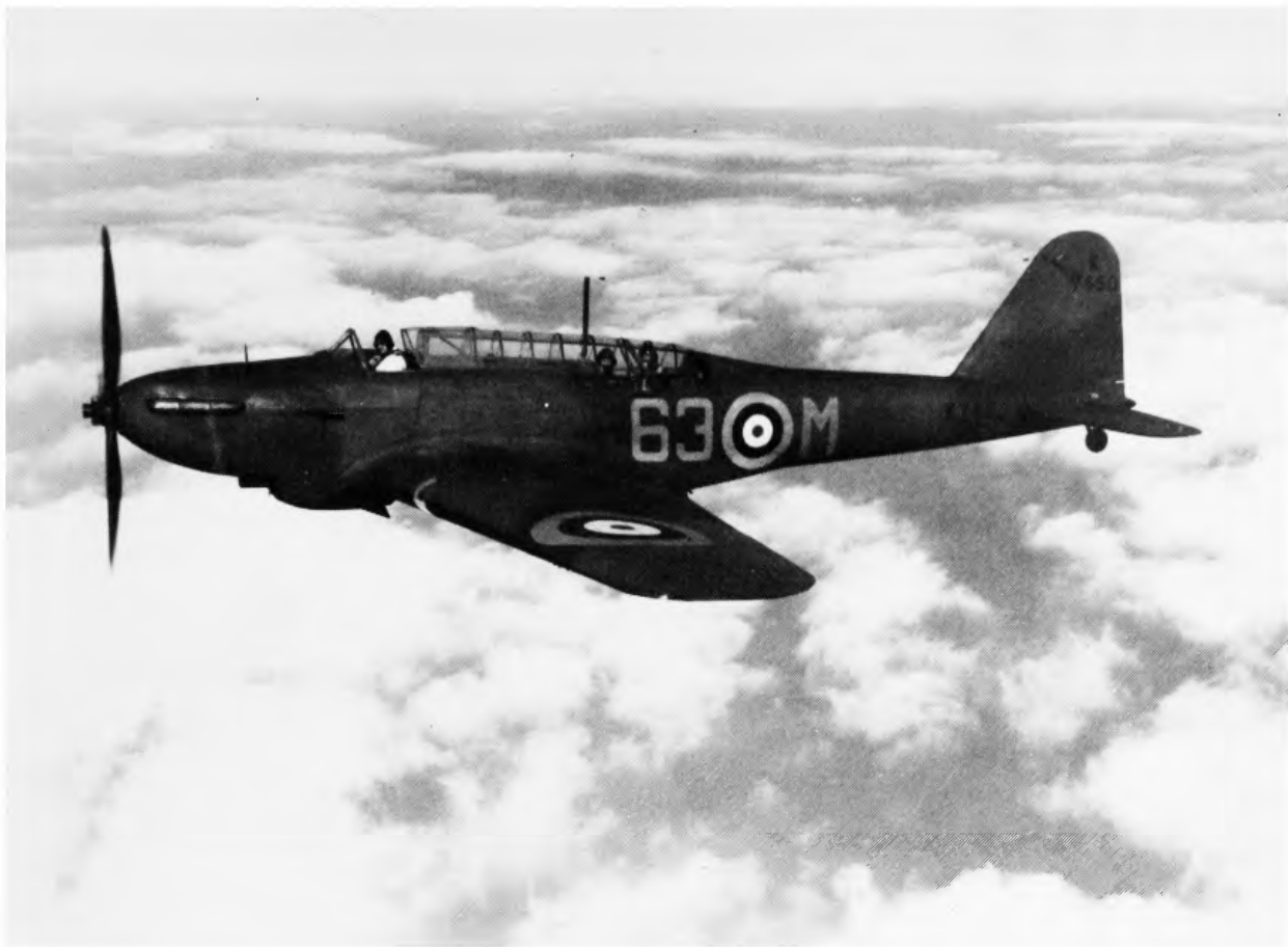
Fairey Battle as used by the AASF in France. Note the lack of defensive armament against attack from below. (RAF Museum).
