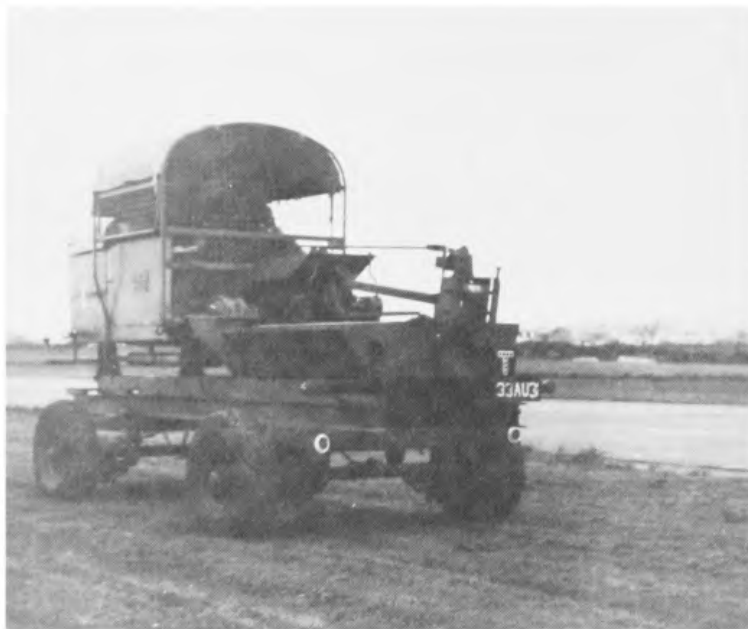
The type of winch (modified balloon winches used during the war) which were used at Hawkinge and were standard equipment with the Air Training Corps.
