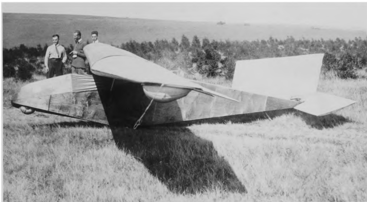
The Vampyr, showing the pneumatic, tricycle undercarriage and the leather cockpit cover which was fastened over the pilot's shoulders, leaving only his head exposed. The pilot here is Hentzen.
