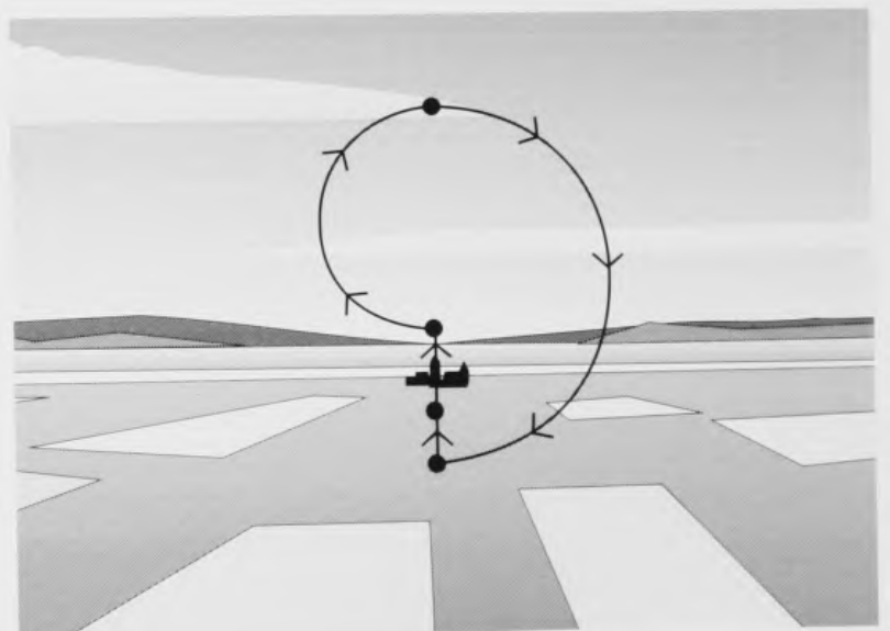
Fig 29 Path Described by Glider Nose during the Full Roll
