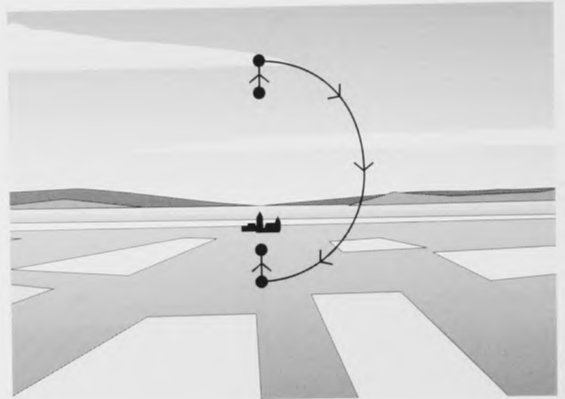
Fig 28: Path Described by Glider Nose Rolling from Inverted to Erect Flight
