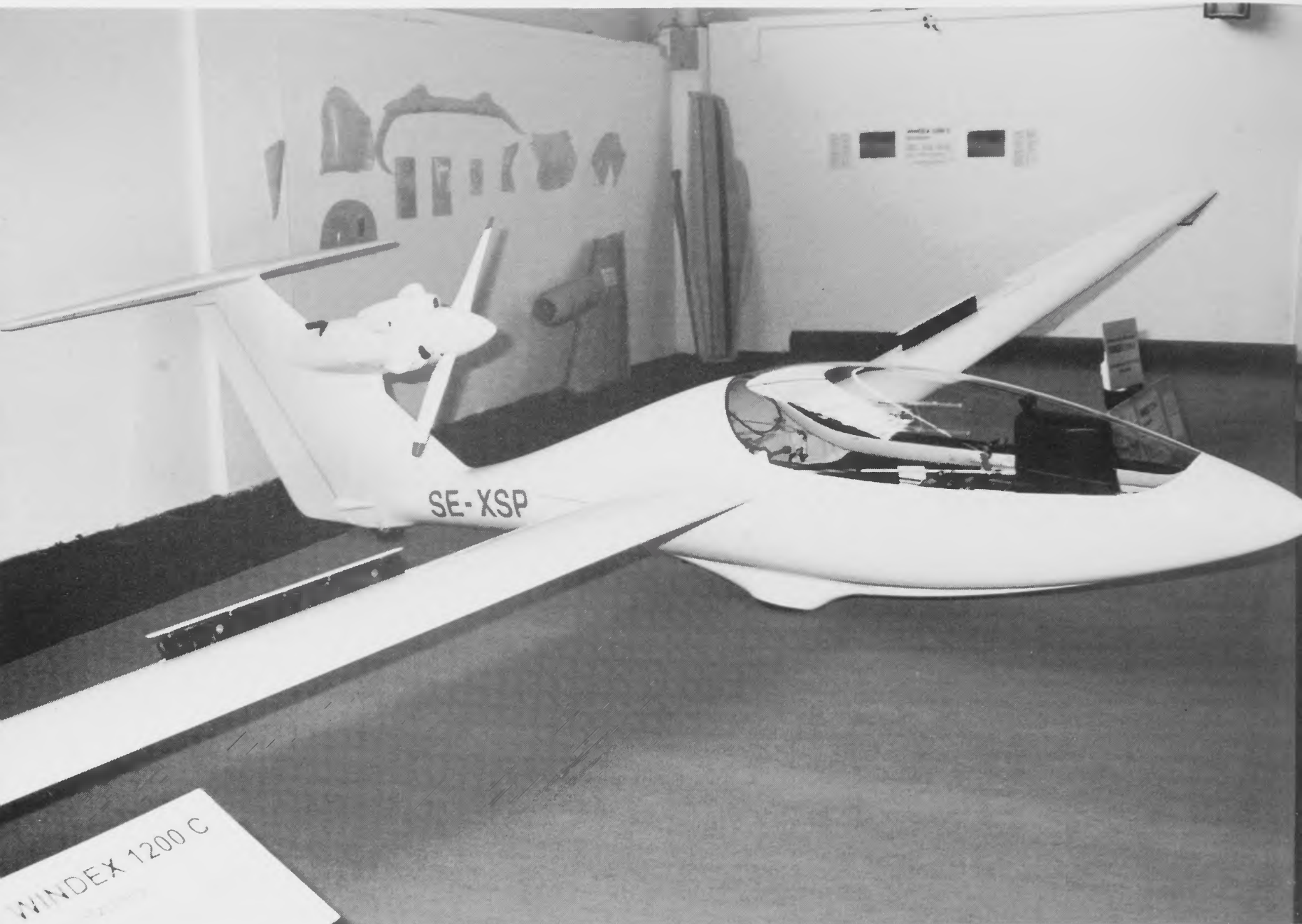
ABOVE: The Windex 1200C fully aerobatic motor glider. ( J. Ewald ) OPPOSITE TOP: The spacious cockpit of the Luňák. ( Mike Woollard ) OPPOSITE BELOW: The prototype Polish Swift S1 'Unlimited' glider, based on original Kobus design. ( Guy Westgate )
