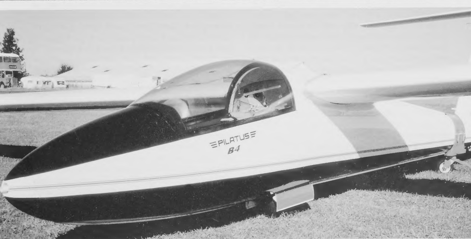
The all-metal Pilatus B4 is an early 'Unlimited' aerobatic glider, outclassed today by the newer Fox, Swift and Celstar designs. (Mike Woollard)
