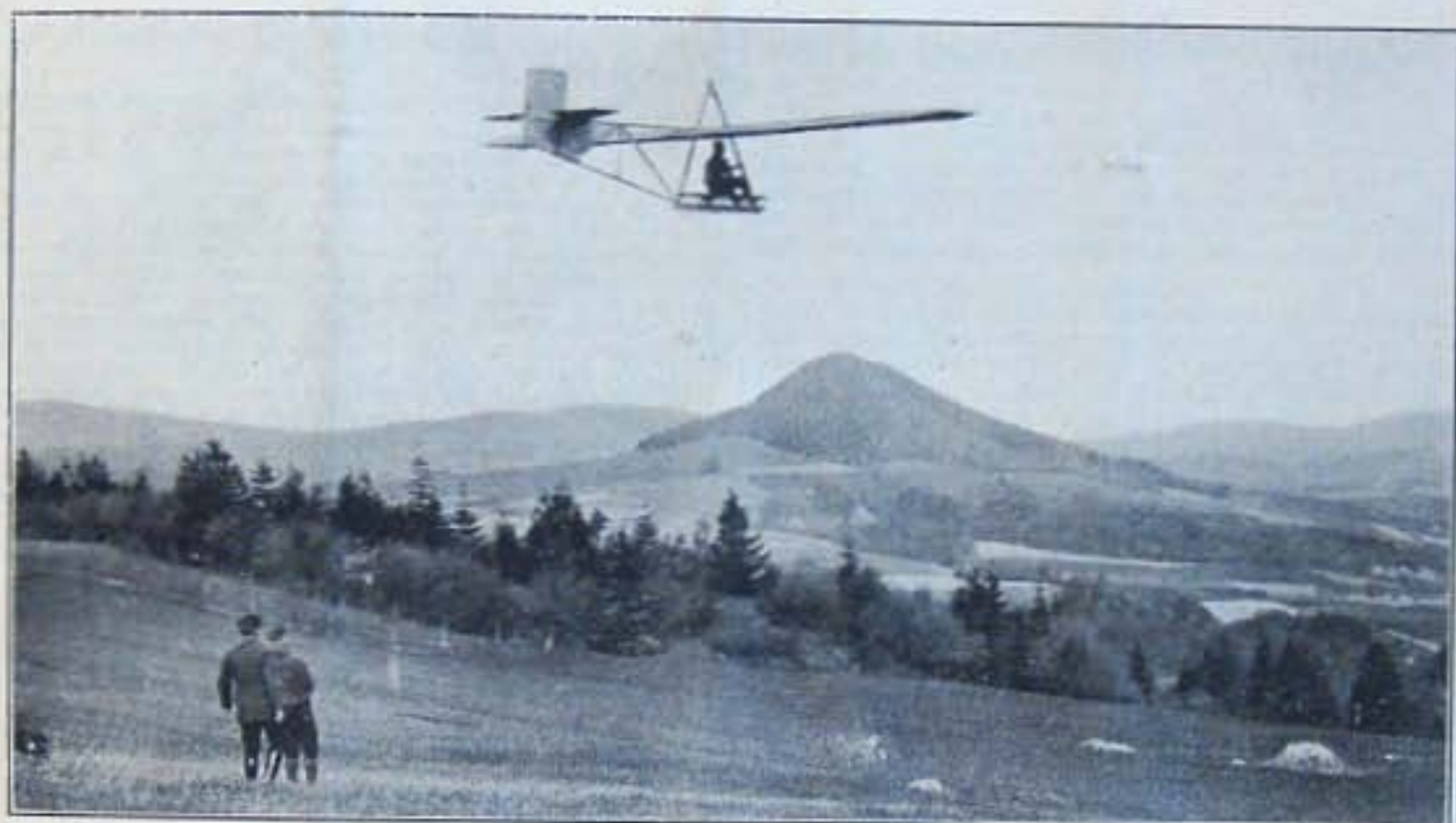
A pupil making a training flight at Grunau, where Wolf Hirth is in charge. The sloping strut in front of the pupil has been known to do more harm than good.
