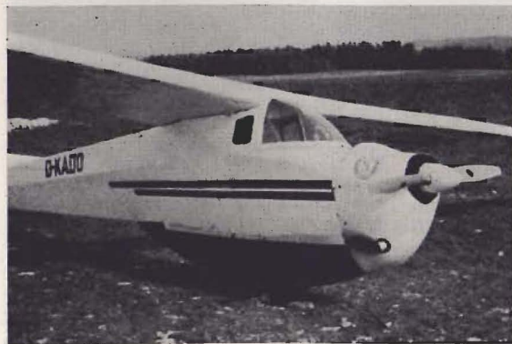
The Wankel rotary engine neatly cowled-in on a Scheibe Motorspatz. There has been for some years a Motorspatz on the UK register fitted with a Hirth 4-cylinder 2-stroke engine. Photo: Peter Ross
