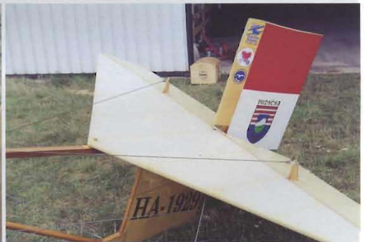
Leather straps hold the pilot's feet on the rudder pedals; instruments are not standard All-moving rudder is too small to compensate for the large amount of aileron drag
