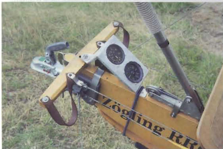
Leather straps hold the pilot's feet on the rudder pedals; instruments are not standard All-moving rudder is too small to compensate for the large amount of aileron drag
