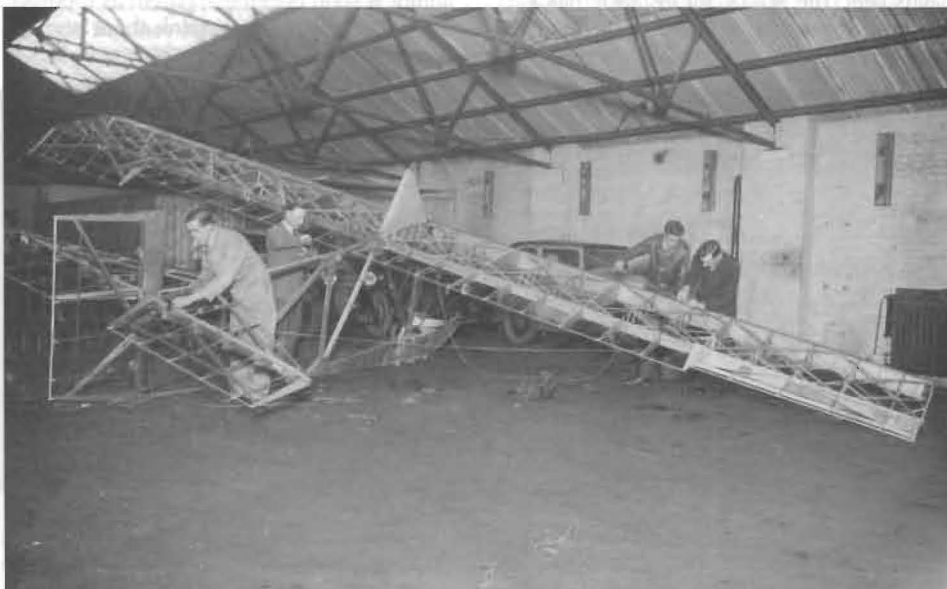
Building a primary glider, almost certainly a Zögling, at Beacon Hill Aerodrome in Essex in 1936
