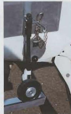
Top, right and opposite: rigging from the purpose-built trailers (Cobra or Komet) can easily be done by one person in ten minutes, says Jochen
