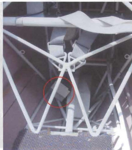
Not the kind of thing you want unsecured in a fuselage: the loose battery jamming the right aileron torque tube
