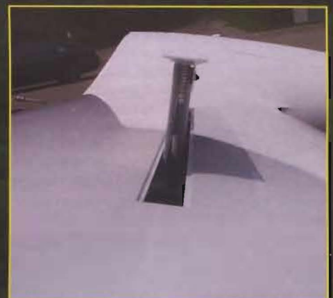
Left: one of the two main pins is inserted into the tongue-tongue spar connection then (inset) locked Above: ILEC engine management controls are well positioned at the very base of the instrument panel Right: Bee's single-bladed Schempp-Hirth airbrakes
