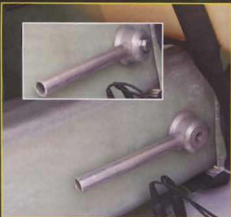
Left: one of the two main pins is inserted into the tongue-tongue spar connection then (inset) locked Above: ILEC engine management controls are well positioned at the very base of the instrument panel Right: Bee's single-bladed Schempp-Hirth airbrakes
