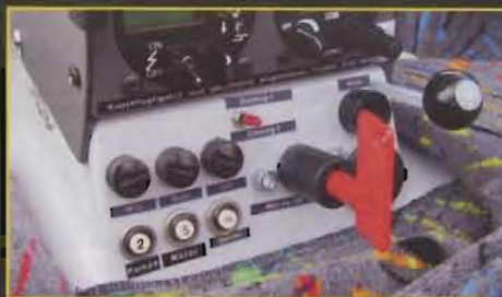
Left: one of the two main pins is inserted into the tongue-tongue spar connection then (inset) locked Above: ILEC engine management controls are well positioned at the very base of the instrument panel Right: Bee's single-bladed Schempp-Hirth airbrakes
